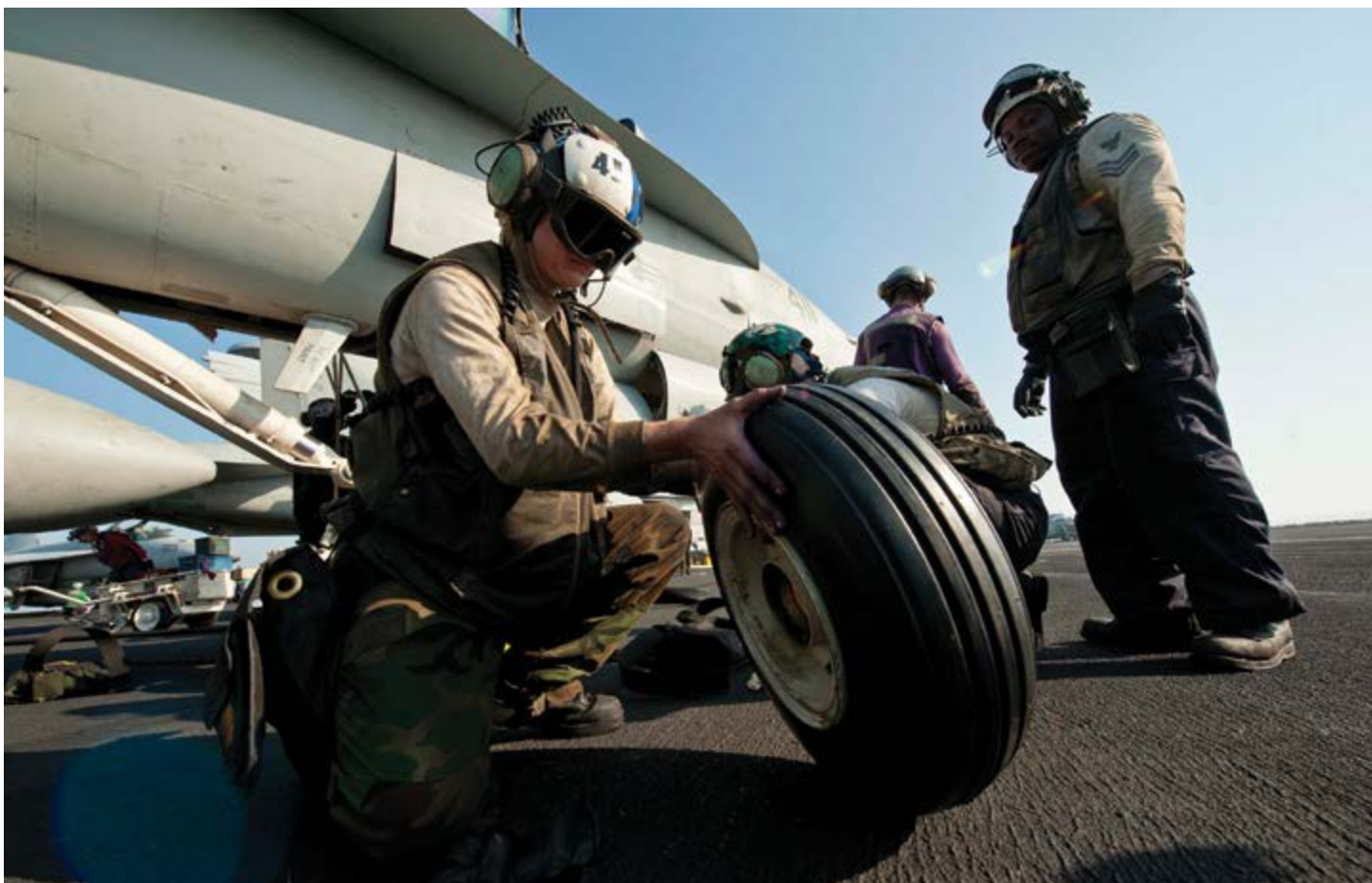
U.S. Navy Aviation Machinist's Mate 2nd Class Catherine Clements inspects a tire before installing it onto an F/A-18C Hornet assigned to the Golden Dragons of Strike Fighter Squadron
