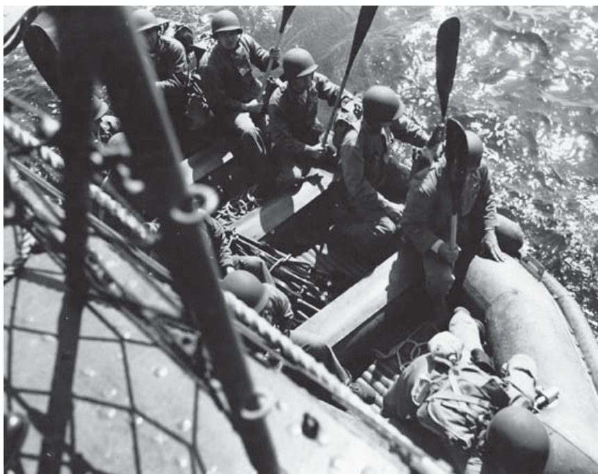
Raiders alongside a destroyer transport prepared to cast off. The paddle blades have been painted matt black to reduce moonlight reflection caused by flashing paddles. Note the bundle of M1 rifles, which were lowered into the boat by rope. The same method would be used to hoist weapons out of the submarines' deck hatches. (Tom Laemlein/Armor Plate Press)
