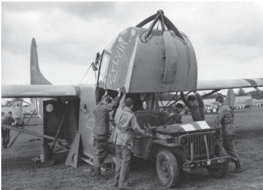
This CG-4A being loaded ready for Operation Market in September 1944 is fitted with the Ludington-Griswold nose and large Cory nose skid. Two support poles prop up the glider’s tail to tip the nose forward to allow easy loading and unloading. The right-side troop door is open, and the triangular kick-out emergency panel under the wing leading edge can be seen leaning against the fuselage. (Tom Laemlein/Armor Plate Press)
