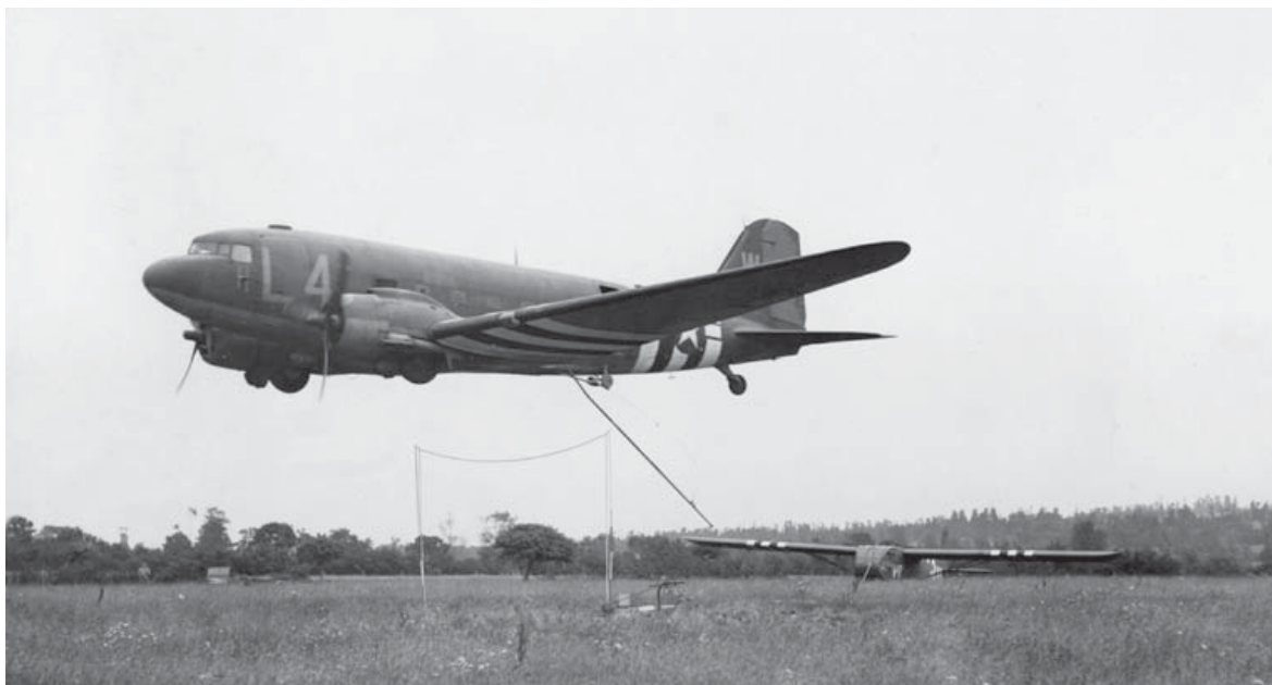
This C-47 painted with invasion stripes is making its run to snatch a CG-4A off a pickup zone. The lowered 20ft hook-arm is about to snag the pickup rope suspended between two "clothesline" poles – see Plate H. (Tom Laemlein/Armor Plate Press)
