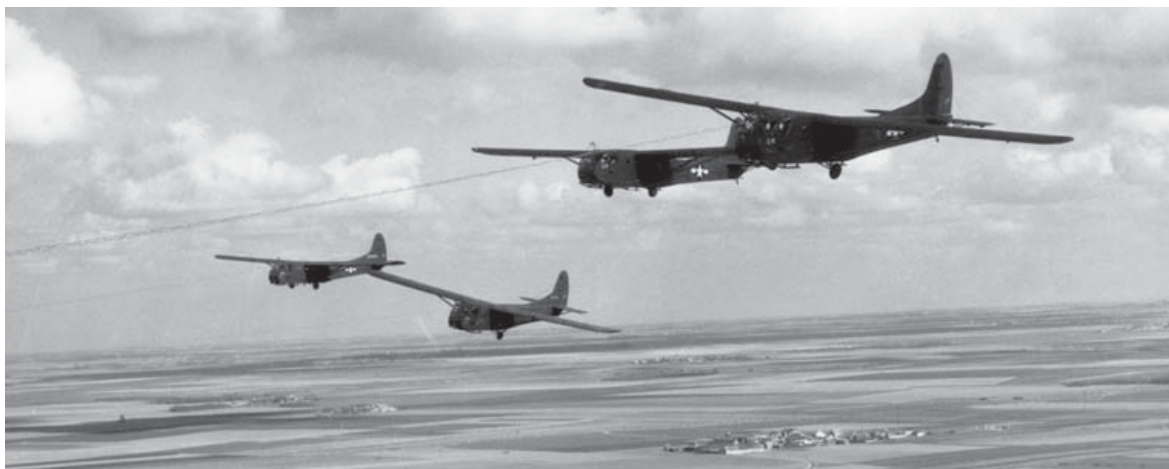
Waco CG-4As under tow by C-47 transports in a tight formation – “a pair of pairs.” Both tug and glider pilots had to pay close attention to relative positioning; a glider swaying around could cut another’s tow-rope. (Tom Laemlein/Armor Plate Press)
