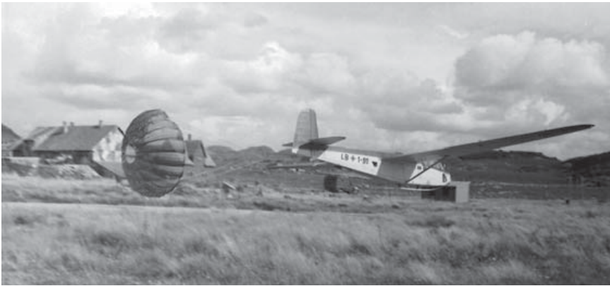
The DFS 230 was designed to make short landings; it could be provided with a drag parachute, as here, which reduced its landing speed by almost half over a short distance. For trials some were even fitted with nose-mounted braking rockets. (Bundesarchiv 1011-568-1531-32)
