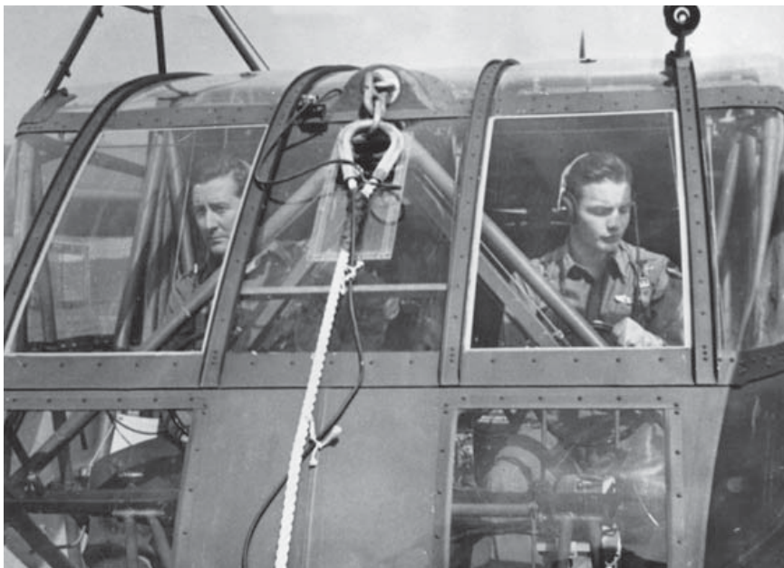
The details of the CG-4A's tow-rope connection; note the telephone cable tied to the rope with slack loops, to allow for tow-rope stretch. (Tom Laemlein/Armor Plate Press)
