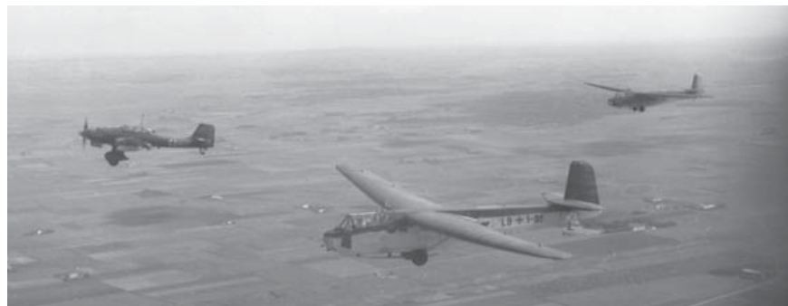
Over Italy, 1943, Junkers Ju 87 dive-bombers tow DSF 230s, here with 100m (330ft) ropes. The Stuka tugs were used for short-range cargo delivery flights, and to tow their own units' mobile workshops fitted in gliders. (Bundesarchiv 1011-567-1523-35A)
