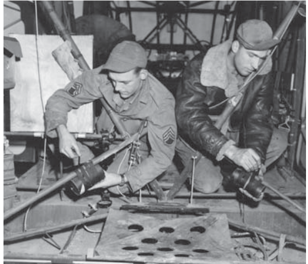
A glider mechanic (left) and pilot tape AN-M14 thermite incendiary grenades to framing struts in a CG-4A. After the troops or cargo have been unloaded on the LZ, the grenades will be ignited to burn the hulk. The pilot wears a dark brown B-3 winter flying jacket and a B-1 summer flying cap. (Tom Laemlein/Armor Plate Press)
