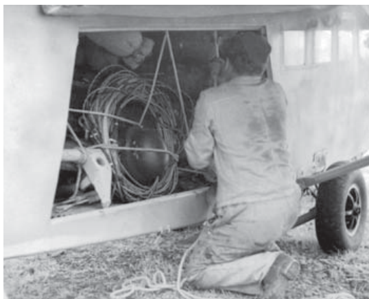
A ground crewman checks the cargo load of a DFS 230. In the Lastensegelflugzeug (cargo glider) role it could carry up to 2,800lb, but the inability to remove the front five centerline seats limited its usefulness, since items had to be crammed in around and on top of these. (Bundesarchiv 1011-565-1407-06A)
