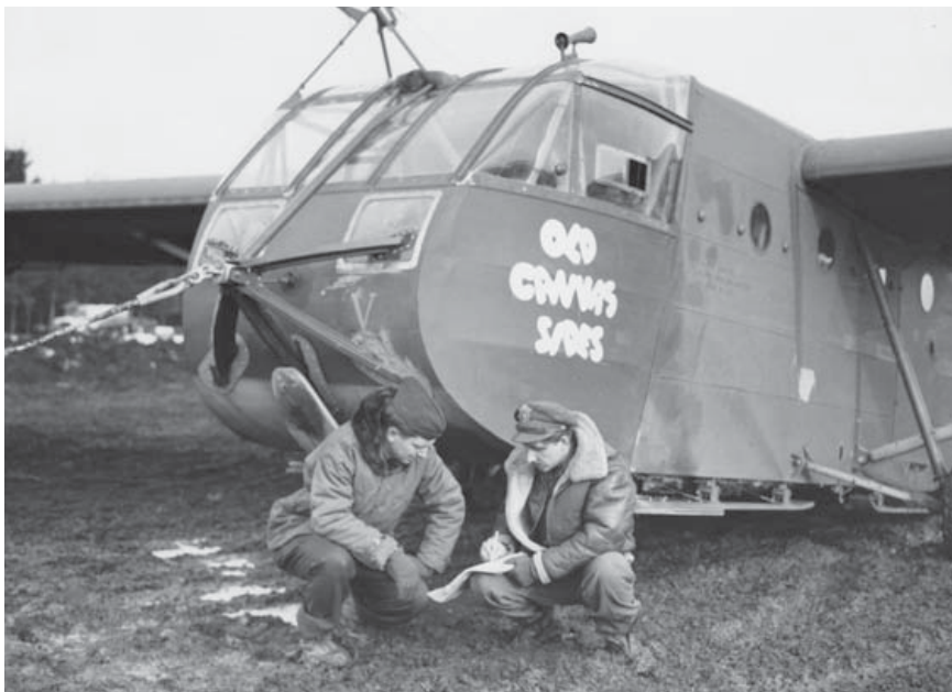
Two IX Troop Carrier Command pilots discuss their mission; their CG-4A is fitted with the Ludington-Griswold nose reinforcement and the wide Cory skid, and the tow-rope is already hitched on. The right-hand pilot wears a dark brown B-6 winter flying jacket while the other wears an olive drab B-11 model. (Tom Laemlein/Armor Plate Press)
