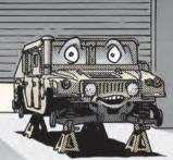
VEHICLE SUPPORT STANDS DO NOT REQUIRE FUNCTIONAL TESTS AS TB 43-0156, SAFETY INSPECTION AND OPERATION OF STAND, VEHICLE SUPPORT, STATES, PERIODIC LOAD TESTING OF JACK STANDS DOES MORE HARM THAN GOOD. IF THE STAND'S BEEN TESTED OR CERTIFIED BY THE MANUFACTURER, THAT'S THE ONLY TESTING IT WILL EVER NEED
