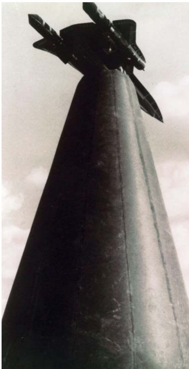
A 1/8th scale A-12 model undertakes RCS testing. The extensions aft of the engine nacelles were added to simulate the aircraft's exhaust plume. (Lockheed Martin)
