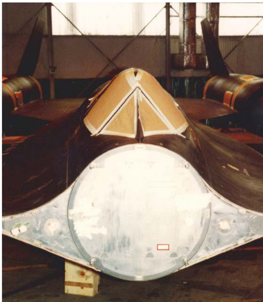
The addition of fuselage chines to the "Blackbird" family's circular forebody transformed its cross-section into a "stealthy" two-dimensional "flying saucer," a discovery made independently by both Frank Rodgers and Ed Lovick. (Paul F. Crickmore)
