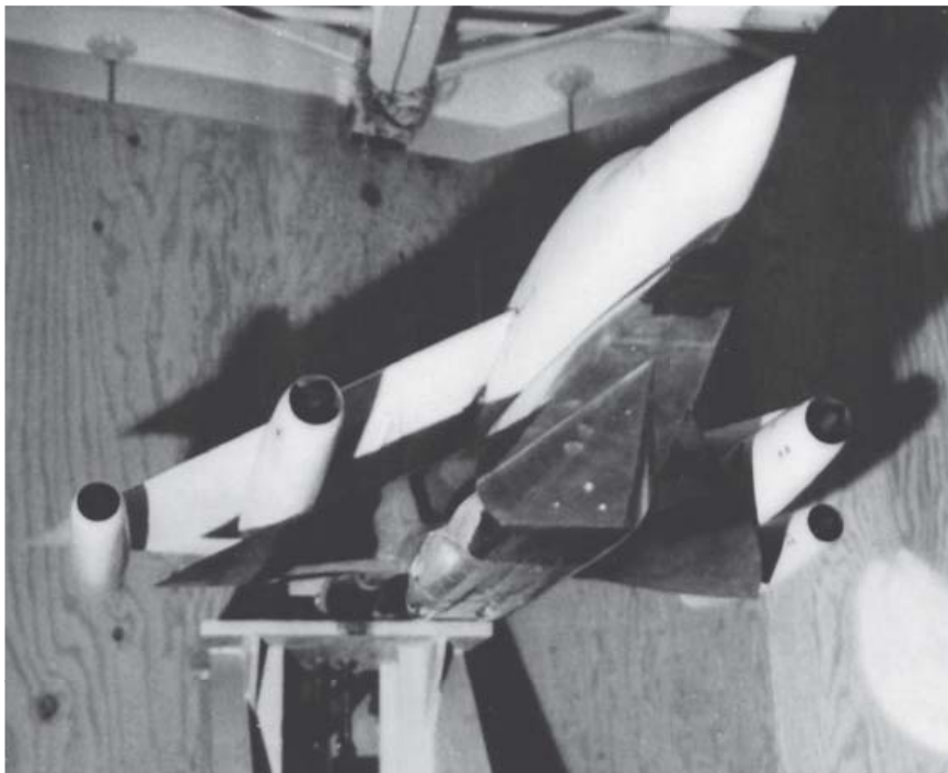
This wind tunnel model shows Convair's FISH concept being carried beneath the underside of its B-58 launch aircraft. (Lockheed Martin)
