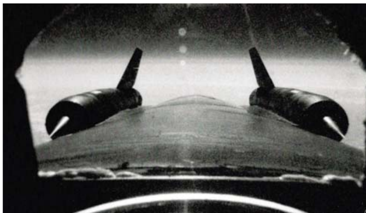
A rearward-facing cine camera was mounted behind the cockpit of the three Black Shield Oxcarts, the idea being to film SA-2 attacks, although it isn't known if any footage was ever captured during at least three of the known incidents. In this picture the aircraft is seen at speed and altitude – note the position of the fully retracted spike to produce the maximum inlet capture area. (Roadrunners Internationale)
