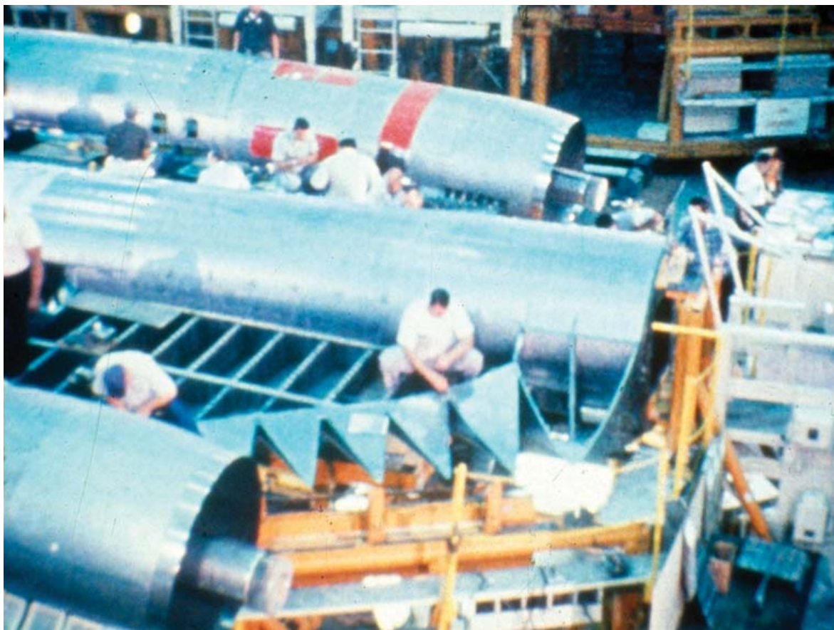
This rare color shot shows engineers within Skunk Works Building 309/310 at Plant B-6, getting ready to position the inboard wing leading-edge serrations onto an A-12. (Lockheed Martin)
