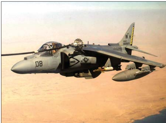
Lt Col Sanborn’s wingman also takes on fuel from a VMGR-452 KC-130T on 22 September 2004 over Lake Tharthar. Most Al Asad-based Harrier IIs were fitted with the General Electric GAU-12U Equalizer 25 mm five-barrel Gatling gun, and its 300-round magazine, in the twin underfuselage pods (US Marine Corps)
