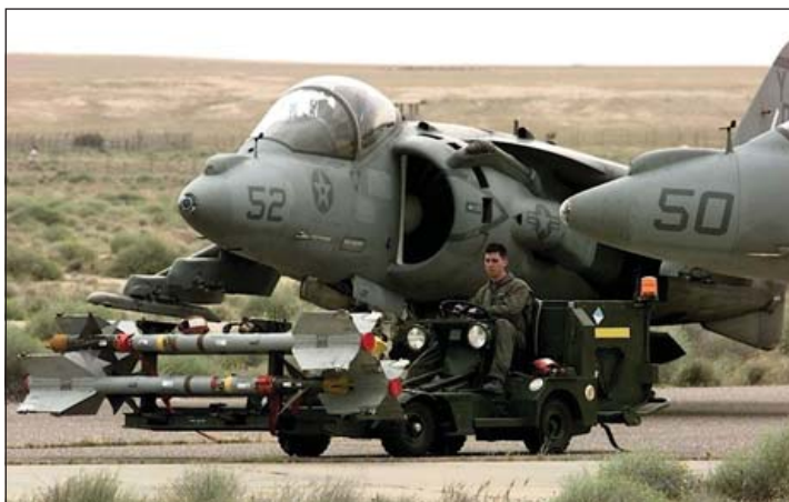
VMA-211 returned to OSW duties in early 1998 when Detachment A went ashore to Ali-Al-Salem from USS Tarawa (LHA-1) while the rest of 11th MEU-SOC/HMM-268 exercised in Kuwait. In this photograph, taken on 29 March 1998, a detachment maintainer has borrowed a USAF missile-loading tractor to transport four AIM-9M Sidewinders out to the VMA-211 dispersal area (US Marine Corps)
