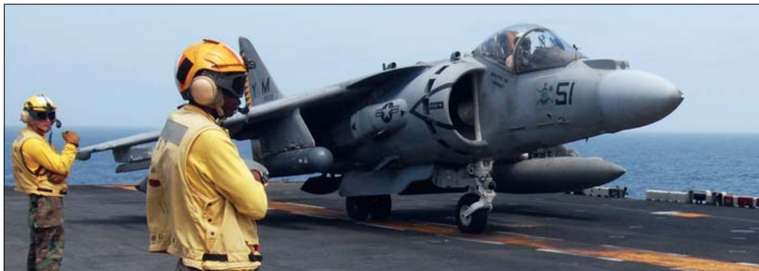
Like VMA-513 'Det A' before it, VMA-542 'Det A' conducted its OIF missions exclusively from the flightdeck of its amphibious assault ship – in this case USS Iwo Jima (LHD-7). This aircraft, awaiting clearance for takeoff in November 2006, is armed with a 500-lb GBU-38 JDAM on its inner port wing pylon (US Navy)
