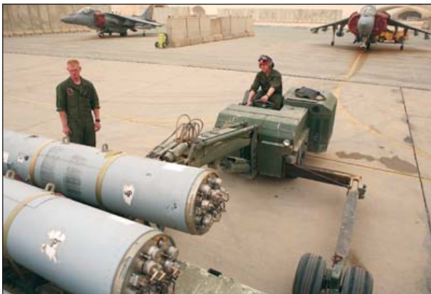
Ordnance Marines of VMA-542 unload SUU-25 flare dispensers from a trailer before moving them over to the AV-8Bs parked behind them on 14 March 2008 at Al Asad. This system was periodically used by Harrier II units in-theatre for battlefield illumination at night (US Marine Corps)
