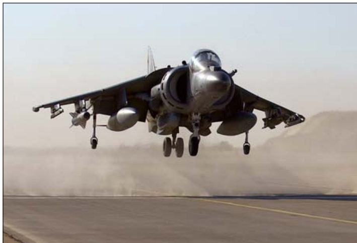
In November 2004 VMA-311 arrived at Al Asad to replace VMA-542. This particular aircraft from the unit, photographed returning from a mission on 7 January 2005, is armed with a GBU-12 and an AGM-65E Laser Maverick. It would almost certainly have been paired up with a Litening II-equipped Harrier II on this sortie (Col Clyde Woltman)
