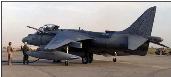
A VMA-214 Harrier II is refuelled by personnel from Marine Wing Support Squadron 271 at a Forward Arming and Refuelling Point (FARP) within Iraq on 3 April 2003. The AV-8B+ is being refuelled ‘hot’, with its engines running. This was just one of many FARPs set up south of Baghdad during the final stages of OIF I. Some made use of recently captured airfields, while others were situated on long stretches of highway (US Marine Corps)
