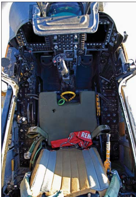
The cockpit of the AV-8B Harrier II+, which includes two Honeywell CRT displays (the non-radar Night Attack aircraft has only one CRT, to the left), a centre-mounted communication-navigation keypad and a Smiths HUD, plus back-up instruments. The Harrier II's Stencil S-III-S SJU-4 ejection seat is also well illustrated from this unusual angle (Ted Carlson/Fotodynamics)
