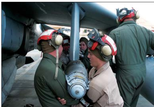
Ordnance technicians of VMA-513 mount a 500-lb GBU-38 JDAM under the wing of an AV-8B on 2 April 2006. The JDAM is a 'fire and forget' weapon, which means that once the target is identified and the GPS coordinates are entered into the bomb's guidance system, the pilot can forget about the target and focus on finding another one. This weapon is not affected by weather conditions, being guided to the ground coordinates set into the system by INS and GPS. On 11 May 2006 VMA-513 delivered the first GBU-38 strike against insurgent positions (US Marine Corps)
