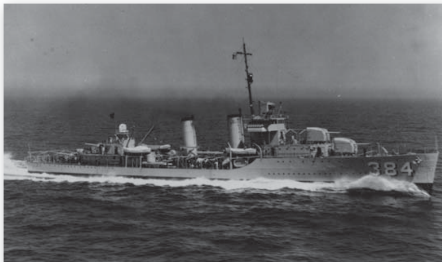
Dunlap (shown here) and Fanning repeated the Mahan design except for the substitution of base-ring mounted 5-inch/.38s forward, protected by fully enclosed gunhouses, and a single pole mast. (NHHC)
