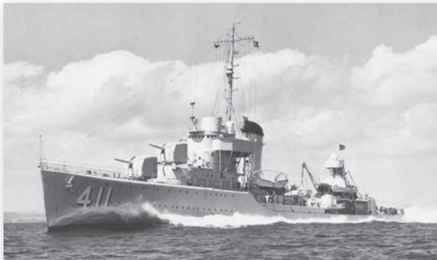
The streamlined Sims class epitomized a transition between an era of shipyards as engine builders and shipyards as assembly facilities, a central theme in the design history of the US Navy's prewar destroyers. Here Anderson , the first to commission, runs builder's acceptance trials in 1939. (NH 96119)
