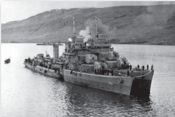
Kearny was first to demonstrate the toughness of American destroyers by surviving a torpedo hit from U-568 on October 17, 1941, before the United States formally entered the war. The damage to her forward fireroom is evident as she lies off Iceland alongside Monssen . (NARA 80-G-28788)
