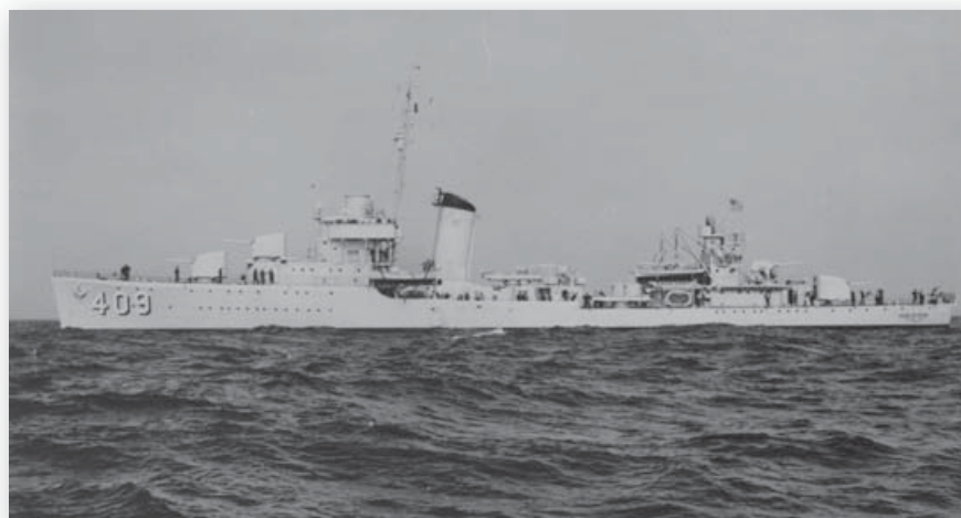
The new Sims , not yet fitted with her main battery director, carries five 5-inch/.38s and 12 tubes: one quadruple mount on the centerline and one on each wing. Characteristic of the prewar period are whaleboats that masked her No. 3. 5-inch gun. (NH 24122)
