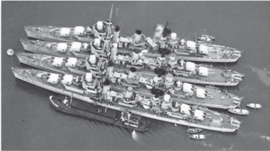
Porter-class 1,850-tonners Balch , Moffett , Winslow , and McDougal , moored at San Diego in 1939, exhibit their single-purpose 5-inch twin mounts and 1.1-inch antiaircraft gun positions fore and aft. (NARA 80-G-422626)
