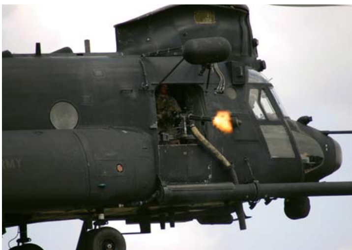
A door-gunner aboard a 160th SOAR MH-47E engages a target with his 7.62×51mm M134 minigun. Electrically powered, these guns were knocked out when RAZOR 01 lost its electrics during the crash landing on Takur Ghar. (DOD)
