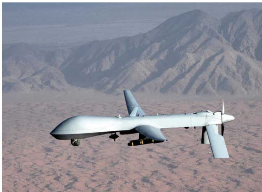
An armed RQ-1 Predator of the type which provided vital close air support to the Rangers. This Predator carries two AGM-114 Hellfire II guided antitank missiles. Recent versions now have the capability to carry a GBU-38 500lb JDAM. (DOD)
