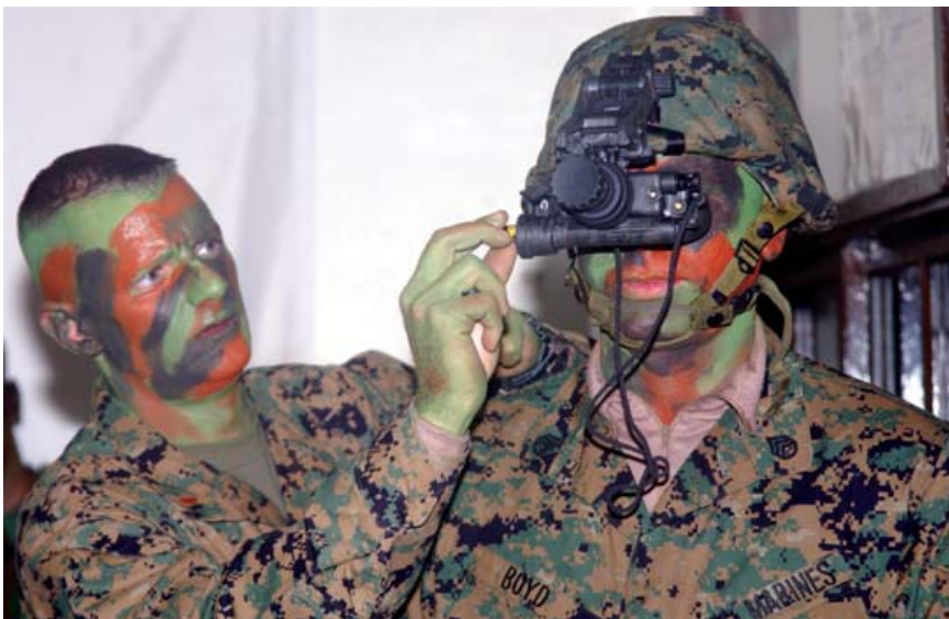
A chief warrant officer demonstrates battery replacement during a 2005 presentation on the use of AN/PVS-7 night vision goggles. (Lance Cpl Cristin K. Bartter/USMC)
