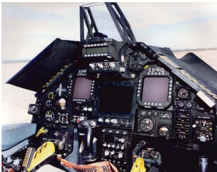
The active liquid crystal display incorporated in the HUD indicates that this is a post-OCIP Phase III F-117 cockpit. (Lockheed Martin)
