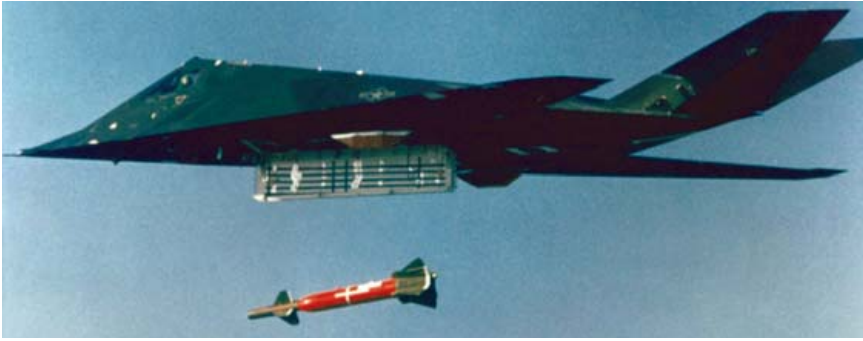
Aircraft 784 is seen here dropping an inert 2,000lb GBU-27 during separation trials. The weapon's release trapeze remained in the bomb bay, to ensure the aircraft retained the lowest possible RCS during the weapon release phase of attack. Note the underwing fairing housing cameras to record weapon separation data. (Lockheed Martin)
