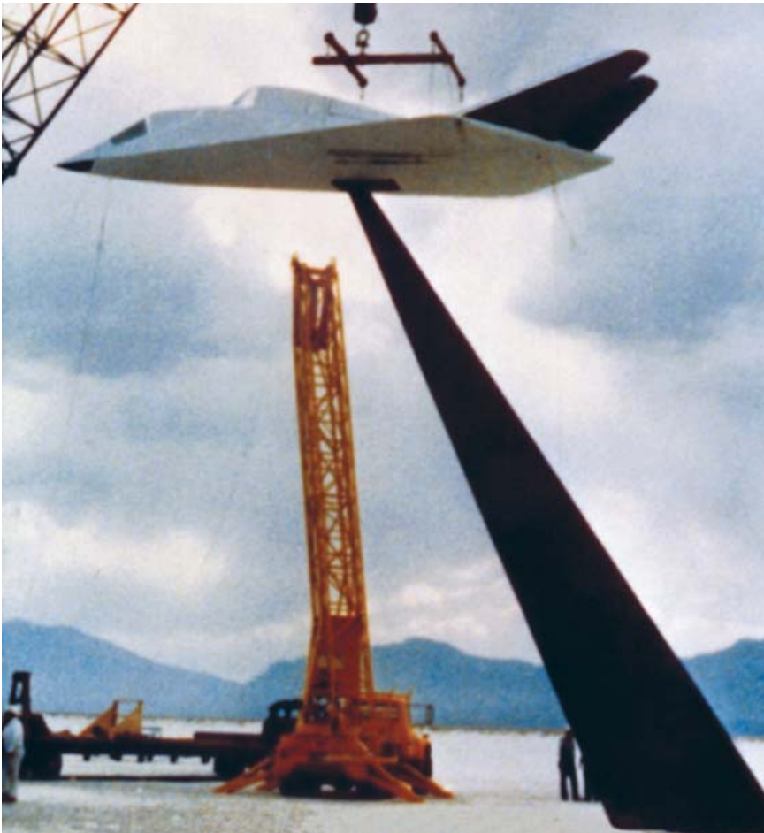
The Northrop full-scale model demonstrator undertaking RCS tests during Phase 1 of the Experimental Survivable Testbed (XST) program at the USAF RATSCAT facility at White Sands, New Mexico in February 1976. (Northrop via Tony Landis)
