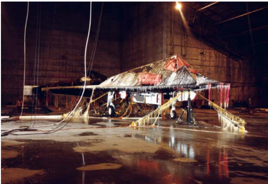
Aircraft 824 underwent a series of climatic tests at Eglin AFB, Florida. It is seen here being brought down to subzero temperatures, having first been sprayed with water. (Lockheed Martin via Tony Landis)
