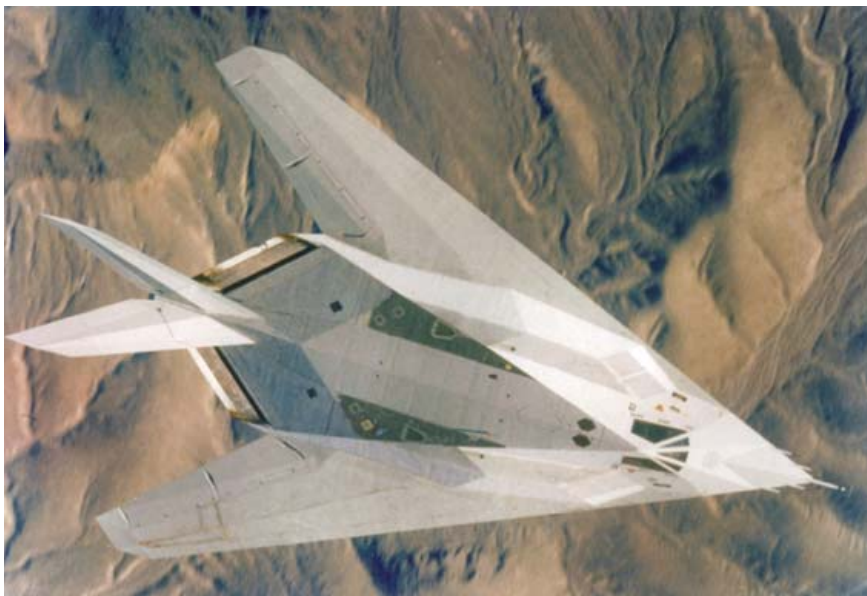
During 780's first period of downtime from August 6, 1981, to October 21, 1981, the aircraft was repainted in an overall, low-visibility gray scheme. The operational fleet was painted black, despite Lockheed's Alan Brown being able to prove scientifically that gray was the best LO scheme for the aircraft. (Lockheed Martin)
