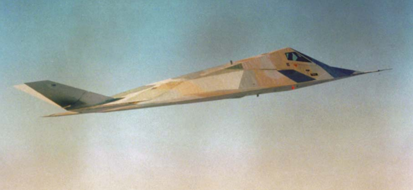
Aircraft 780 sported a unique camouflage paint scheme during the first ten flights of its test program. Note the large test instrumentation nose boom. (Lockheed Martin)
