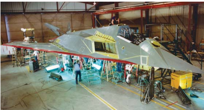
Upon delivery from Burbank via C-5 Galaxy to Area 51 on January 17, 1981, the prototype F-117 (Aircraft 780) underwent reassembly and a detailed checkout of all onboard systems. It made its first flight five months later. (Lockheed Martin)
